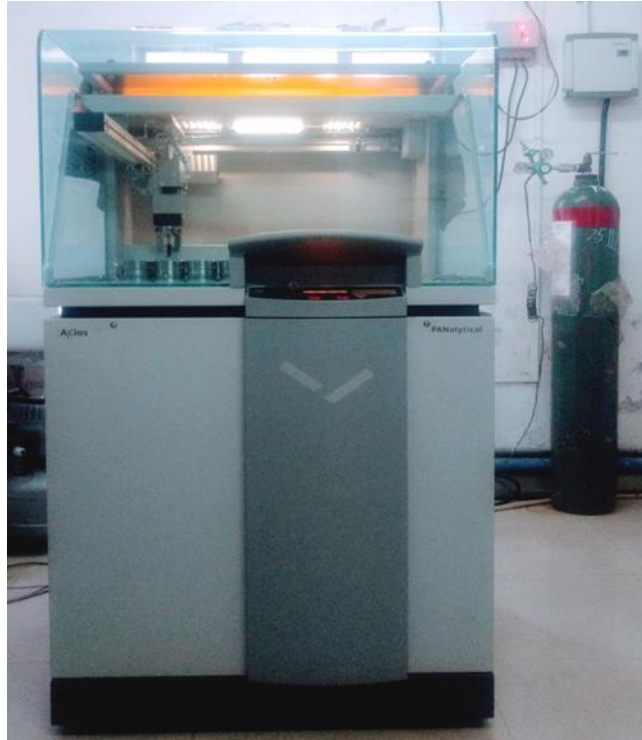
Figure 4.1: X-ray fluorescence spectrometer for soil analysis.
