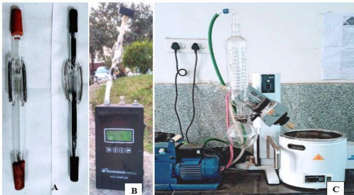
Figure 2.14: [A] Charcoal tube or VOCs sampling tube. Both empty [L.H.S.] and activated charcoal filled [R.H.S.] tubes are shown side by side; [B] VOC sampler and [C] Rotary vacuum evaporator to concentrate the VOC extract in CS 2 solution.
