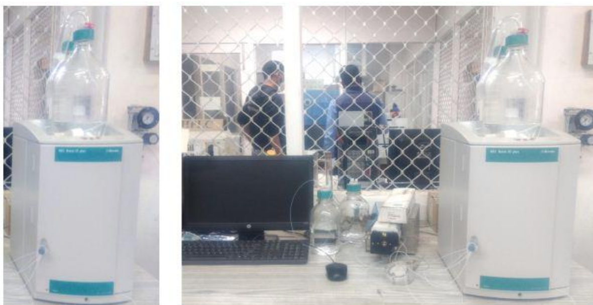
Figure 2.17: Ion-chromatography for poly-atomic ions measurement.
